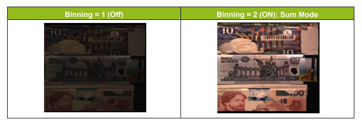
This camera supports Horizontal x2 digital binning on the FPGA.
